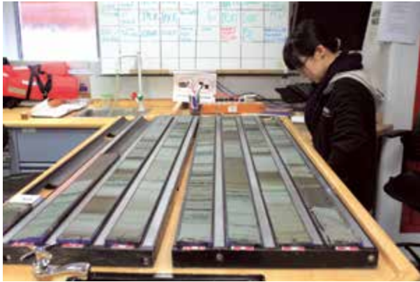
Figure 5.6 A Sea of Japan sediment core showing alternations of dark-coloured (i.e. anoxic condition) and light-coloured (oxygenated) sediment layers. © Ryuji Tada.
